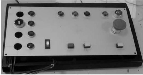
Fig. 6. Real prototype according to the operational modes of the GEMMA guide.
