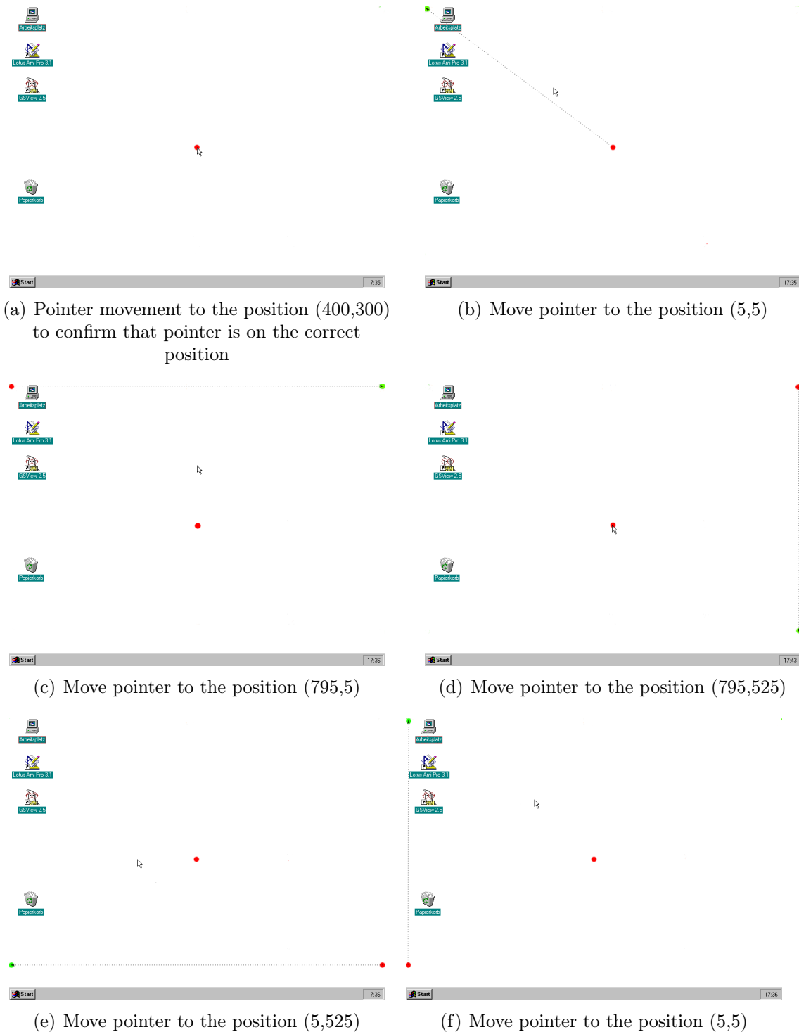
Figure 3.3: Pointer movements sent according to the second set of positions in the Test data with the screen resolution of 800x600 pixels. Screenshots taken from the OS – Windows 95.
