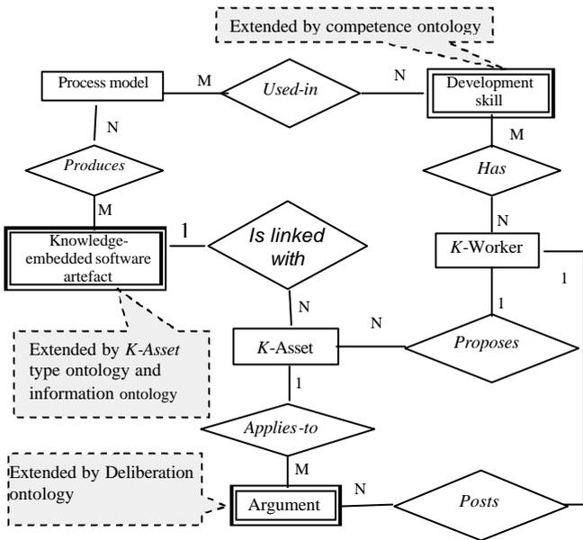
Figure 1. LiSER's knowledge model (higher level domain ontology).
