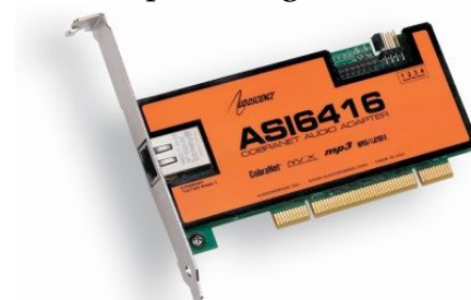
Audio card equipped with Ethernet connector
